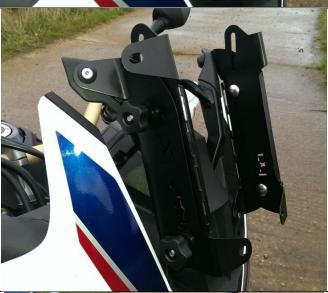
Loosely mount the bracket assemblies to the fairing using the new fasteners provided.
