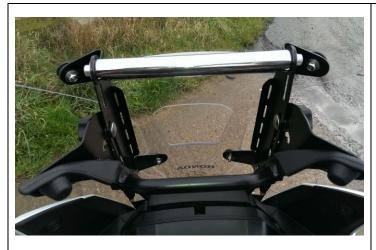
Pre-assemble screen fasteners and retain to screen with rubber washer on the inside of the screen – this makes it easier when fitting to brackets.
