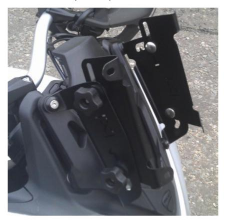
Next, loosely mount the bracket assemblies as shown above, ensuring a plastic washer (provided) is placed underneath each bracket tab.
