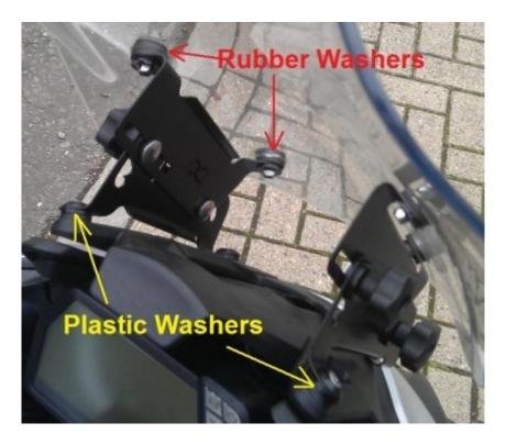
With the brackets in position, loosely mount the screen, adding the lock-nuts and washers provided. Ensure a rubber isolating washer is placed between each bracket tab and the screen - this helps relieve stress on the screen. Finally, tighten the fasteners further, checking alignment of the screen and brackets as you do so.
