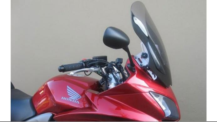
The Varadero/CBF Screen Adapter Kit comes pre-assembled so after the bike's screen is removed, the bracketry can be simply bolted to the existing hole positions in the fairing using the new fasteners provided (note, these have plastic finishing washers).
