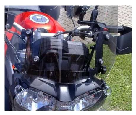
TAKE CARE NOT TO OVERTIGHTEN AS THIS MAY CAUSE CRACKS IN THE SCREEN.
