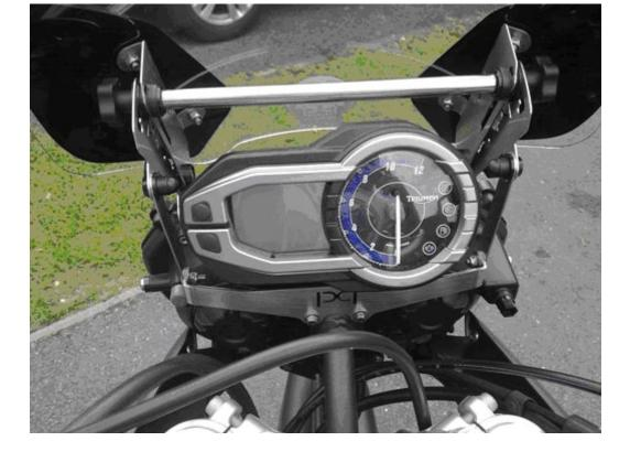
Mount the side bracket assemblies loosely onto the front bracket end hole locations.
