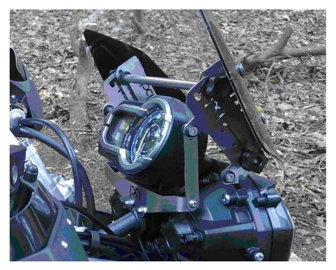
Remove the standard screen and plastic side supports.
