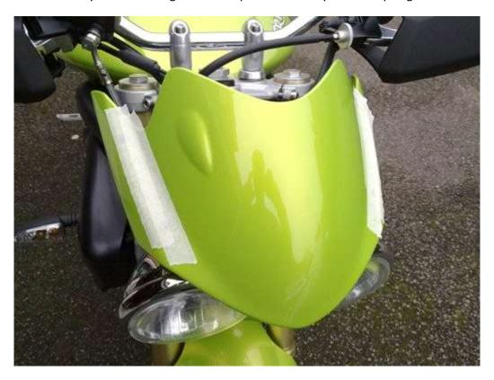
First, apply masking tape either side of the cowl as shown, to allow you to mark the desired hole locations.
