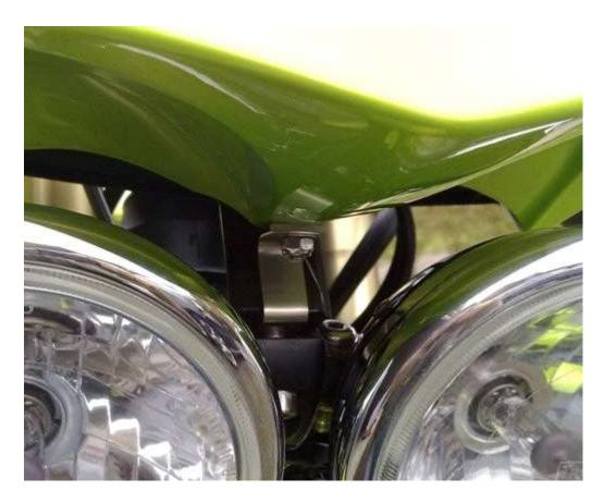
Refit the cowl, taking care to locate the bracket in line with the front clamp bolt and reinsert the bolt.
