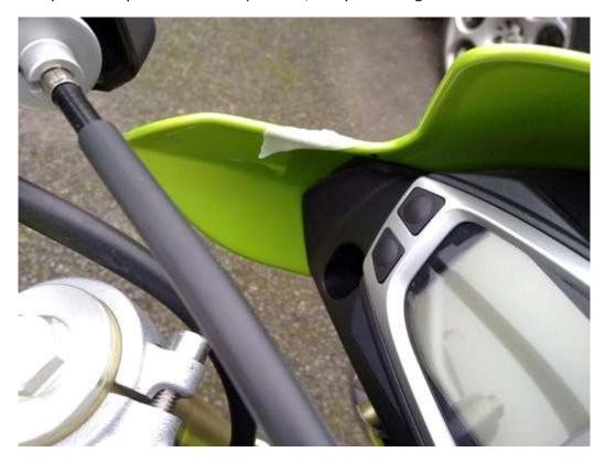
Before removing the cowl to drill the holes, mark where the outside edge (on both sides) meets the cowl - you will need this location to apply two foam pads.
