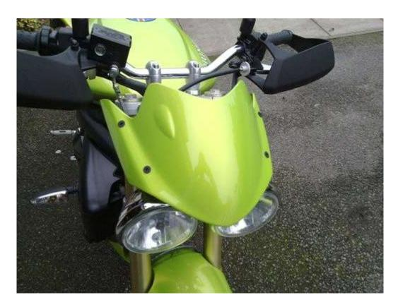
Refit the three cowl/bevel fasteners then install the four rubber threaded inserts.
