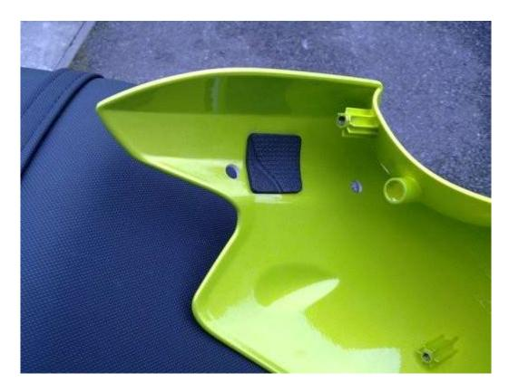
Remove the cowl and carefully drill the four hole positions - it is best to pre-drill the holes with a couple of smaller bits before finishing with the correct 9.5mm drill.
