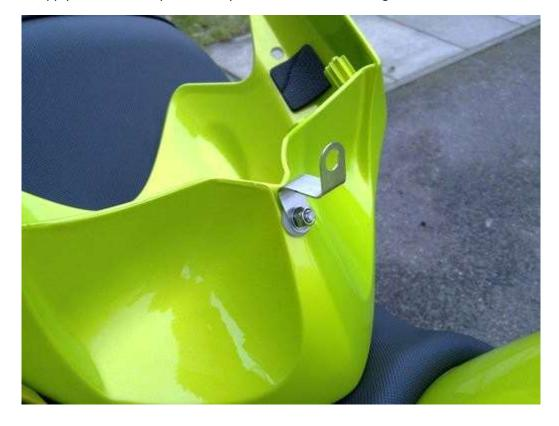
An additional support bracket will need to be fitted to improve the rigidity of the cowl.
