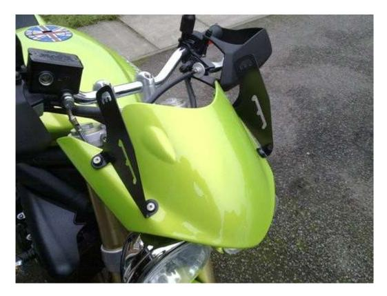
Loosely fit both brackets and recheck their spacing (should be approximately 240-245mm apart).
