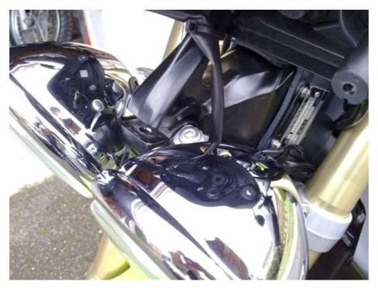
Before loosening the lamp clamp, mark the position of the lights so they can replaced in the same position later.
