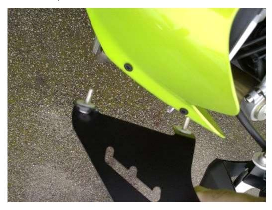
Attach the base brackets using the M5 fasteners provided - making sure a finishing washer is fitted under the head and a nylong washer is attached on the underside, as shown.
