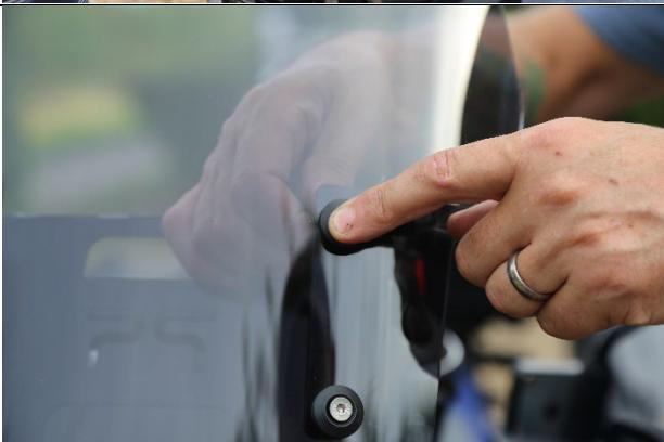
Loosely fit the washers and locknuts. Once everything is aligned, lightly tighten until rubber washers are compressed lightly.
