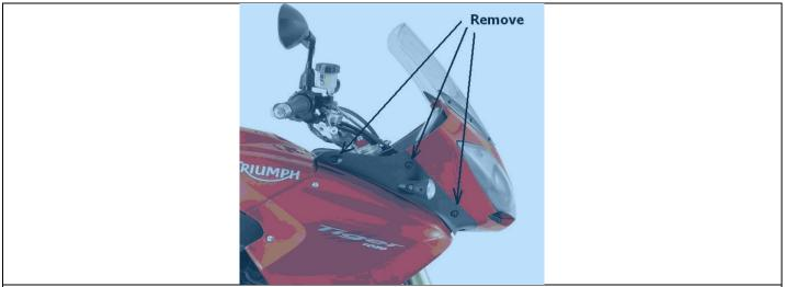
The two screws provided need to be secured with the thread protruding outside the panel to allow attachment of the brace slot - ensure a washer is either side of the brace before securing the plastic knob - these need to be loosened to allow adjustment of the screen brackets.
