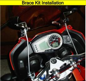
Before drilling the two 6mm holes, check the position you have marked have some clearance on the inside for the screw head - the cowl panels will need to be removed for drilling.
