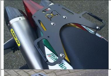
Align the trim with the pillars to check they all align correctly, making minor adjustments to the long pillars as necessary and now they can be fully tightened.
