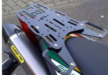
The base-rack will also accept a tail-rack or luggage-rack as shown - ensure the plastic spacers are installed underneath so there is a gap between the two racks as shown.
