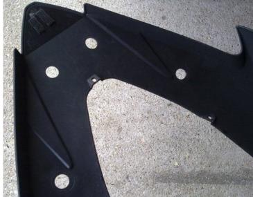
Drill out the four holes in the plastic trim as shown using an 18mm cutter (suitable for plastic) - the hole centres are moulded into the part.
