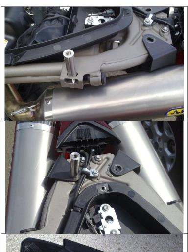
Firstly, remove the plastic tail trim to reveal the rear sub-frame.
