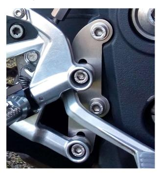
Remove the existing gear-lever and push on the new linkage arm as shown.
