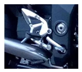
Mount the new drop-plates using the new M8x20 Cap-Head bolts and washers supplied - Torque to 10-12Nm (assuming the threads are in good condition and not been previously over-torqued).
