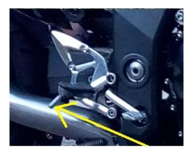
Final step is the bend the side-stand access bar - using a piece of long (300mm+), place it over the arm all the way down to the weld joint and gently bend the arm outwards (small amounts at a time) until the side-stand can be retracted onto its rubber-stopper without interfering with the gear-shift arm.
