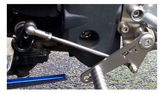
Remove the rear brake arm pin & bracket assembly and insert the new hex connector as shown, fitting a lock-nut either side.
