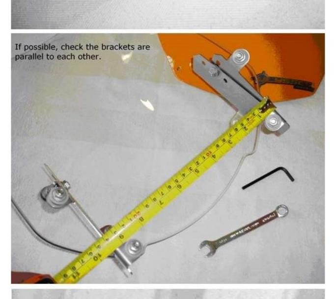
It is important to check that the bracket tabs are parallel with the screen you are using before fastening - the tabs can be bent to provide exactly the right angle if necessary.
