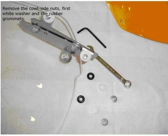
Install the grommets into the cowl.
