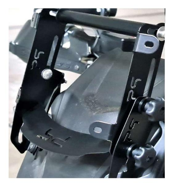
If you have selected the Accessory Bar option, then that mounts onto the top slots as shown above, making sure the plastic washers are placed btween the bar and the brackets.
