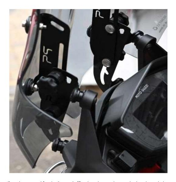
If you have opted for the Screen Baffle, than that can be attached as shown below by loosening the lower fasteners and slotting in position, making sure the square section of the coach bolts (if you have chosen the tool-less adjusters) are correctly seated in the baffle tabs.
