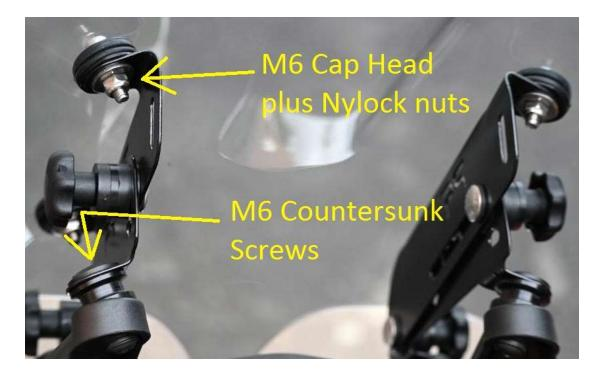
Before tightening, check the left and right hand brackets are parallel and are approximately 150mm apart.
