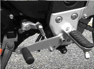
Separate the other Joint in the same way then unscrew the Ball-Connector from the Lever.
