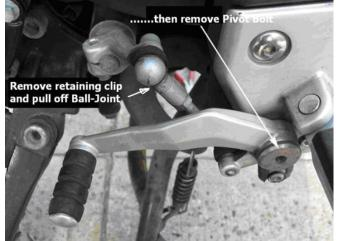
First Step is to remove existing assembly.
