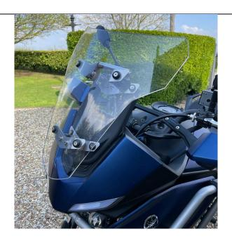
Once everything is aligned, lightly tighten the bracket and screen fixings.
