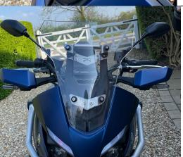
Pre-assemble screen fasteners and retain to screen with rubber washer on the inside of the screen – this makes it easier when fitting to brackets.
