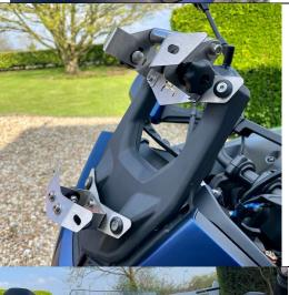
Loosely mount the bracket assemblies to the fairing using the new fasteners provided.
