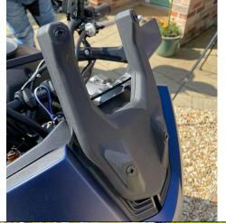
The first step is to remove the original screen fitted to your bike.
