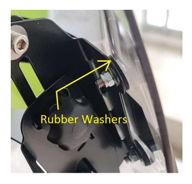
Install the screen onto the brackets and fasten using the washers and locknuts – only tighten just enough to very lightly compress the rubber washers. Overtightening may cause cracks in the screen.
