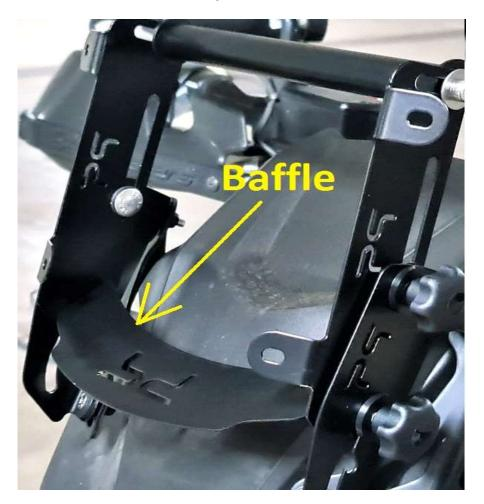
Please note, the Screen's performance is optimised with the Baffle fully open and can be rotated slightly to help fine-tune the airflow required or fully closed to help prevent rain/snow from affecting any electrical items mounted on the Accessory Bar or hitting the rider.
