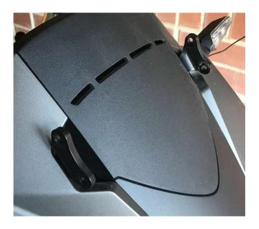
Loosely fit the bracket assemblies as shown and fasten using the screws, washers and lock-nuts provided - ensure the screen brackets are fixed on the inside of the existing base brackets.
