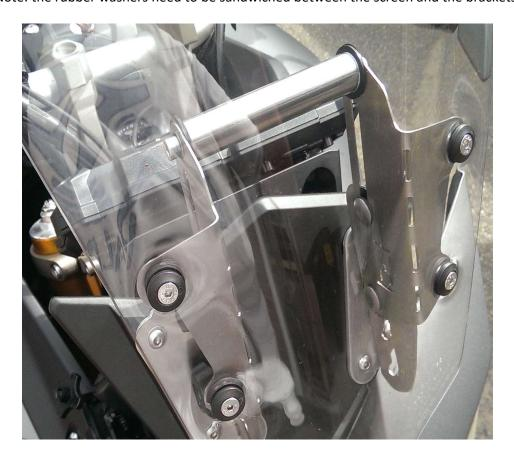
Install the Accessory Bar (optional) as shown in the picture and tighten enough to prevent rotation of the devise you are mounting.
