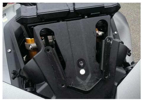
Remove the Screen from the bike and set the mounting brackets in their lowest position.
