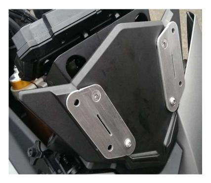
Refit the plastic-cover using the new base-plates and their fixings and tighten to 6-8Nm.
