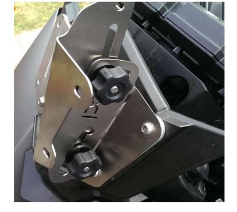
Loosely fit the bracket assemblies as shown and fasten underneath using the long thin washer plate and lock-nuts using around 2-3Nm – do not overtighten.
