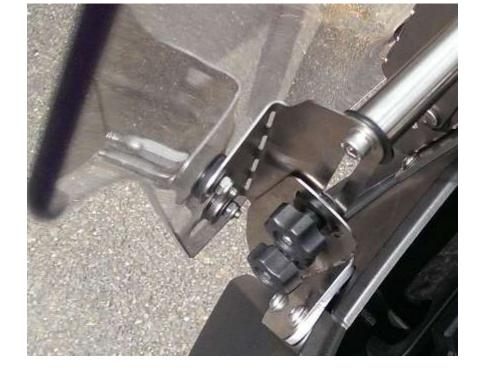
Assemble the new screen screws onto the screen and hold them in place on the back-side using the rubber washers.
