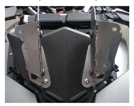
Before tightening, check the brackets are parallel – approx. 100mm apart.
