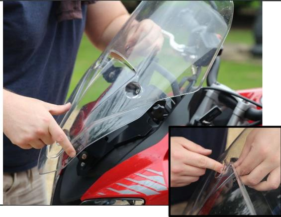
Pre-assemble screen fasteners and retain to screen with rubber washer on the inside of the screen – this makes it easier when fitting to brackets.
