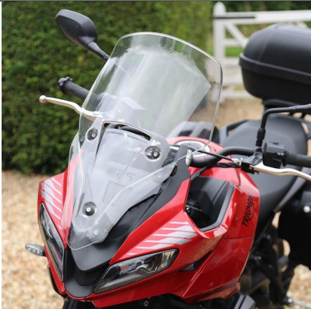
Once everything has been aligned, lightly tighten the bracket and screen fixings.
