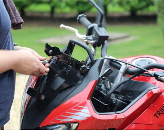
The first step is to remove the original screen fitted to your bike and loosely mount the bracket assembly using the fasteners provided.
